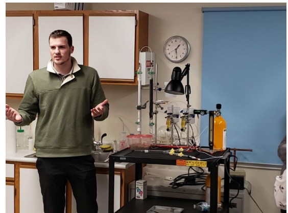
Quinn Kelley demonstrating a Y-tube test which helps determine the attractiveness of different compounds to insects.
