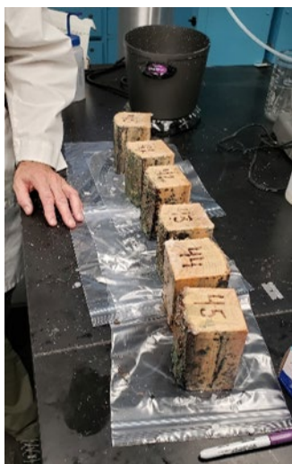
Waxed wood blocks ready for testing by USDA-APHIS
